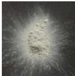
Dry mortar with 0.4 % ARBOCEL® ZCC 500-66 LD
