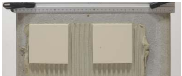
Slipping test for cement tile adhesive
